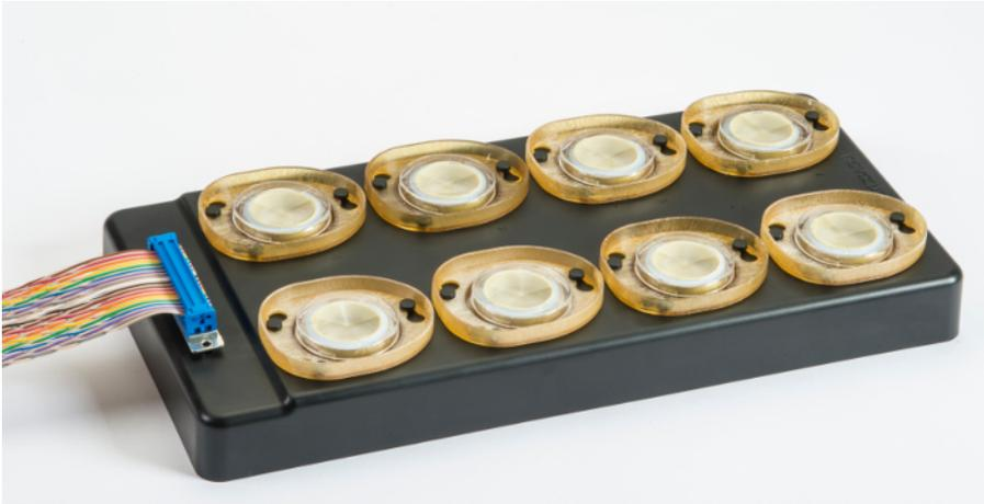
**Figure 1.** TTFields dishes were installed onto a base plate unit and connected to the flat TTFields control cable. [Please click here to view a larger version of this figure.](#)
